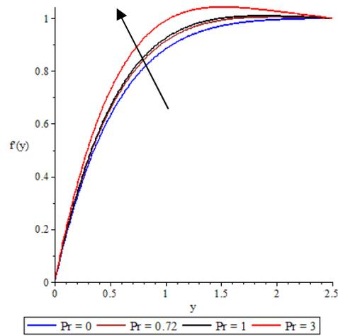
**Figure 4:** Variation of velocity profile for various values of  $Pr$  when  $A=M=\Lambda=Q=Ec=1$  and  $f_0=0.2$
