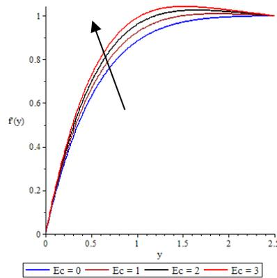
**Figure 8:** Variation of velocity profile for various values of  $Ec$  when  $A=M=\Lambda=Pr=Q=1$  and  $f_o=0.2$
