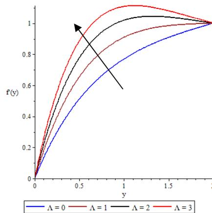
**Figure 7:** Variation of velocity profile for various values of  $\Lambda$  when  $A=M=Pr=Q=Ec=1$  and  $f_o=0.2$
