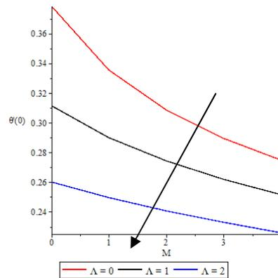
**Figure 19:** Variation of Nusselt number with  $M$  in the present of various values of  $\Lambda$  of when  $A=Q=Pr=Ec=1$  and  $f_o=0.2$
