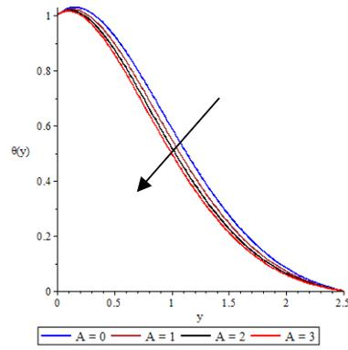
**Figure 9:** Variation of Temperature profiles for various values of  $A$  when  $M = \Lambda = Q = Pr = Ec = 1$  and  $f_o = 0.2$
