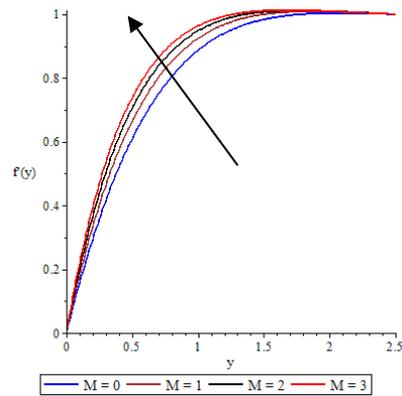
**Figure 3:** Variation of velocity profiles for various values of  $M$  when  $A=Pr=\Lambda=Q=Ec=1$  and  $f_0=0.2$
